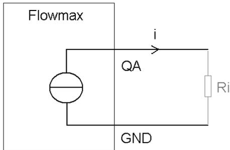
Figure 12: The current output is active
