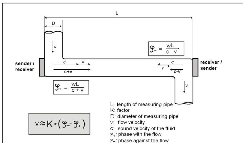
Figure 1: Presentation of the principle of ultrasonic flow measuring
