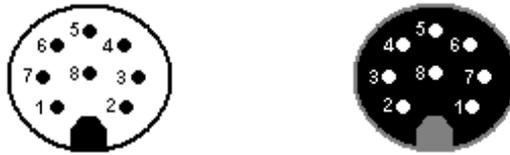
Figure 5: Pin code: Connection plug / socket for 8-pin version
