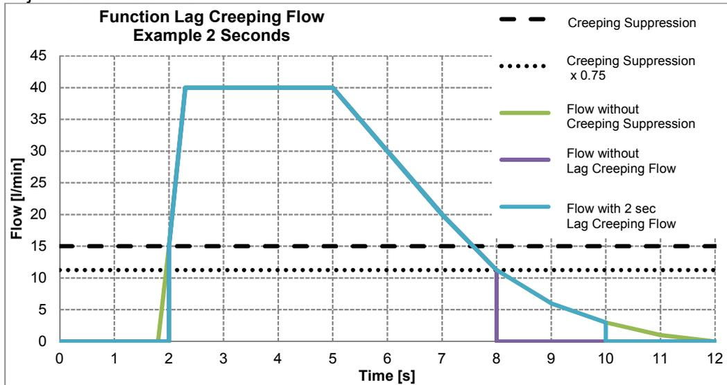
Figure 10: Function Lag Creeping Flow at 15l/min
