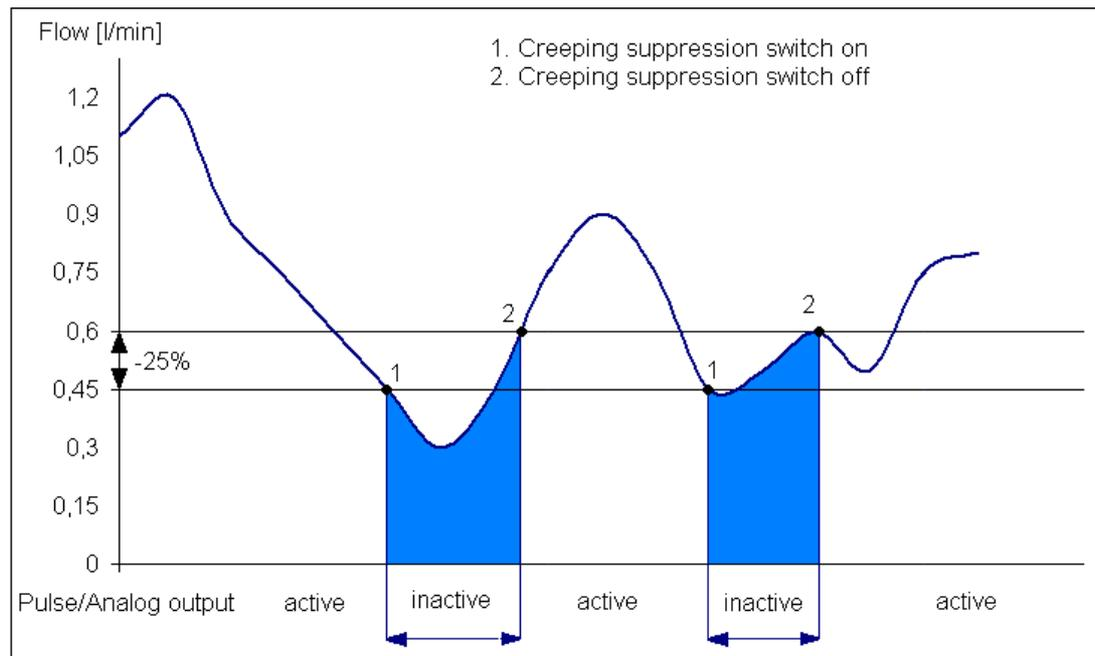
Figure 9: Function of creeping suppression illustrated with 0.6 l/min
