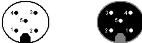
Figure 4: Pin code: Connection plug / socket for 5-pin version
