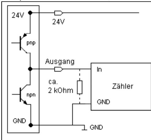
Figure 17: Connecting Digital Output to counter
