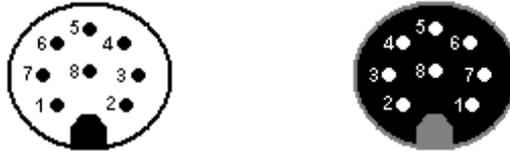
Figure 6: Pin code: Connection plug / socket for 8-pin version
